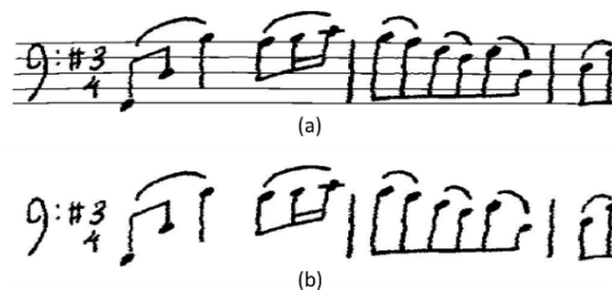
Fig.1. Example of staff line removal in a music score image (a) before and (b) after staff line removal
